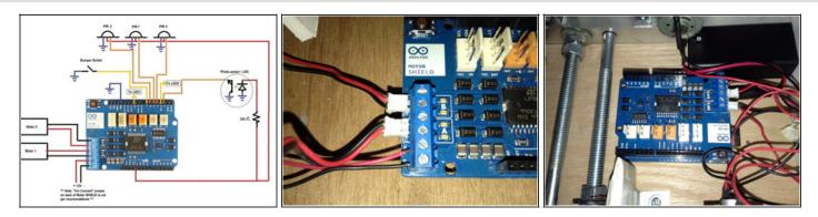
Note: The Arduino Web Page suggests cutting the "V<sub>in</sub> Connect" jumper on the back of the motor shield board when using more than 9 volts. Refer to the Arduino web site for more information.
